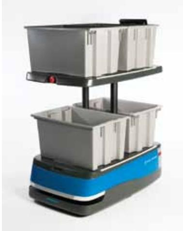
6 River Systems calls its autonomous robot Chuck, which is built from the same technology and sensors as autonomous vehicles.
