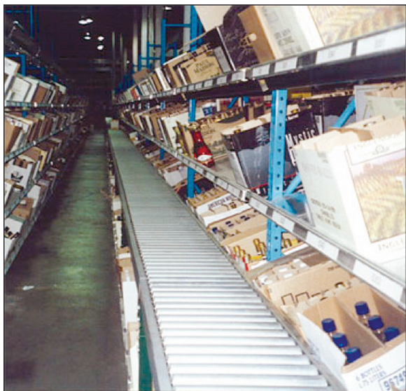
High Velocity Pick Zones concentrate the fast-moving, frequently-touched SKUs in a single area — maybe even its own picking zone.
